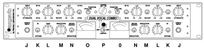
The Dual Vocal Combo has 2 channels which are mirror images of each other and is further divided into top and bottom sections which correspond to the Mic Pre with EQ and the Opto-Limiter Sections. Don't let the mirror image aspect confuse you!
